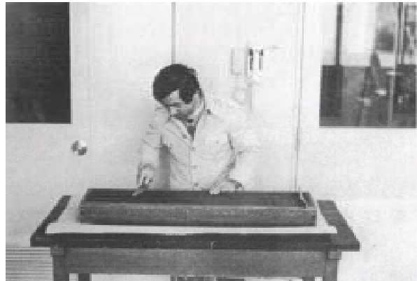
写真-12 削地境：水分調整を行い、表面を平らにする。 Phot. 12. After preparing the moist condition, the profile is again smoothed with a kitchen knife.
