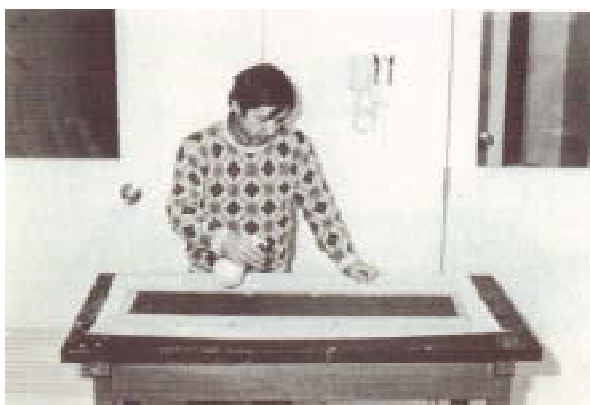
写真-21 濡れ色を出すために，樹脂を感湿する。 Phot. 21. Finally, the soil pool is sensized with a diluted solution of transparent resin.
