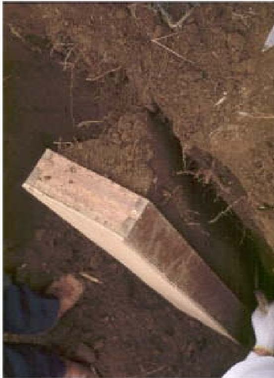
写真-7 土柱の奥にくさび形の切り込みを入れ、スコップを押し込み、手前に開くと亀裂ができる。 Phot. 7. The soil material behind the box is removed, and then the shovel is pushed into the joint part.
