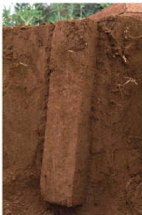
写真-5 断面を掘りこんで土柱を厚きださせる。 Phot. 5. A column of soil with dimensions as the internal ones of the box, is cut in the wall.
