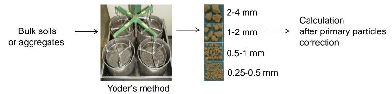
2. Dispersibility test from measuring dispersed particles after shaking
